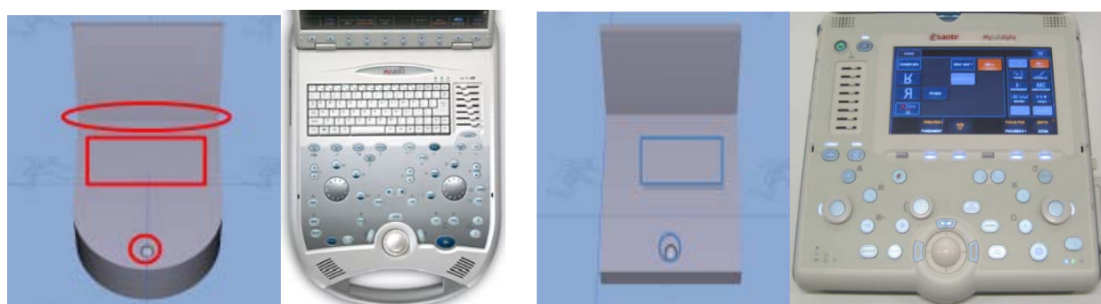
Figure 5: On the left: MyLab30CV Console presented as a simplified .obj model imported in the Santos environment, and a picture of the real interface is presented. In red are showed the different areas of investigations for the simulation conditions of the Left Hand. On the Right: The MyLabAlpha console presented as a simplified .obj model imported in the Santos environment, and a picture of the real interface. In this case, the zones objects of the simulations are showed in blue on the left
